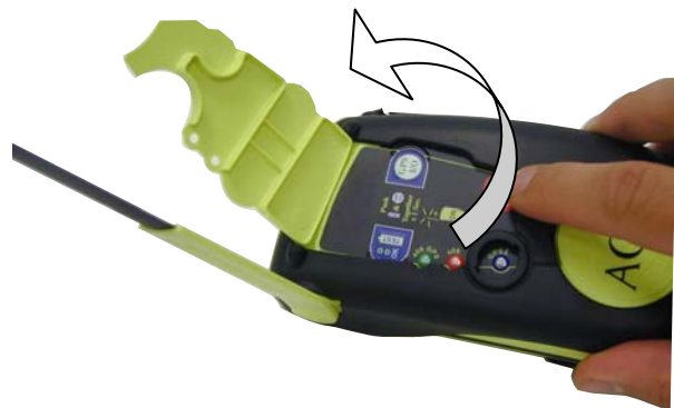
Figure 3 Key pad cover Open the key pad cover for access to Test or activate the beacon
